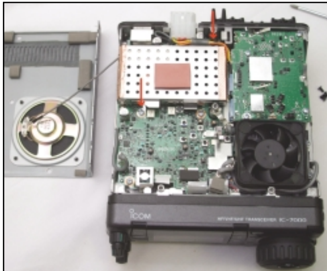
Photo B— Arrows point to the two screws holding the CPU/DSP module in place. Step 3 requires their removal. Step 4 requires the removal of the module.
